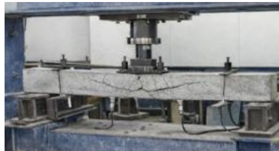
Figure 10 Testing of RC beams
